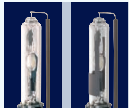
S-type: The cut-off line is created by a shield (left). R-type: To generate the cut-off line in the light distribution a black coating is applied directly on the outer bulb of the lamp (right).
