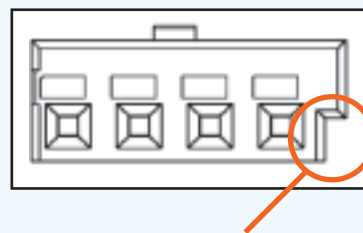
D3-Connector: M-Coding – contact pins Gold-plated
